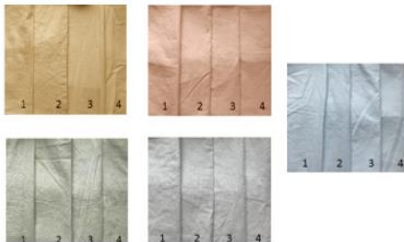
Figure 3. Fabric images after washing (number 1: before washing, number 2: after 1 wash, number 3: after 5 wash, number 4: after 10 wash).
