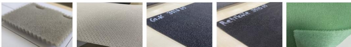
Figure 1. PU lamination foam, perforated PU lamination foam, open-cell PU-based foam, reticulated PU-based foam, multiknit PET- based nonwoven.
