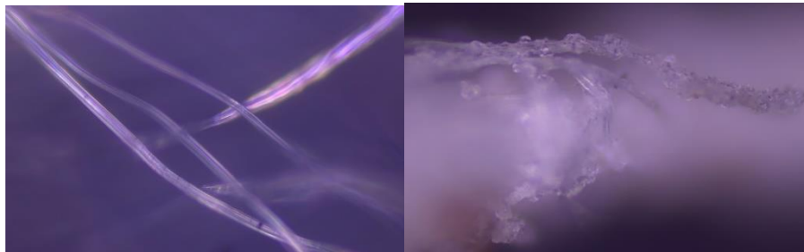
Figure 3. Microscope image of viscon yarn before and after burial in soil.
