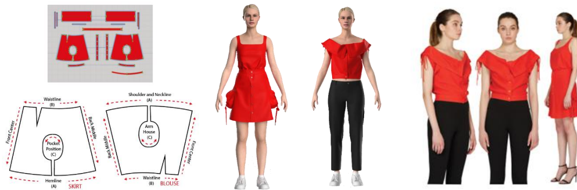
Figure 3: Boat Collar Blouse/ A-Line Skirt (Patterns, Technical Drawing, 3D Simulations, View of the Produced Design on the Mannequin)
