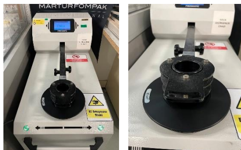
Figure 3. Air permeability machine.
