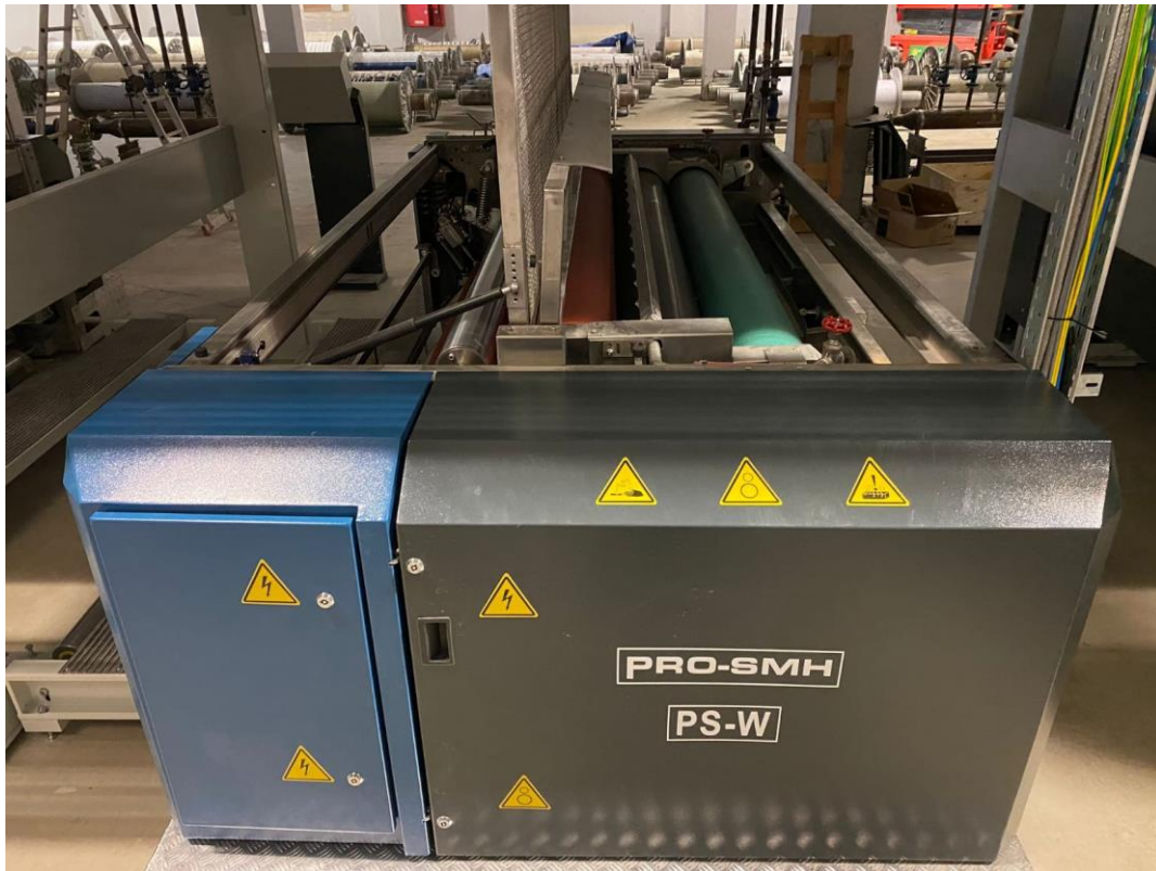
Figure 5. Prewetting application at size box.
