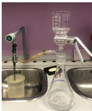
Figure 1. Filtration process for separation of MFs.
