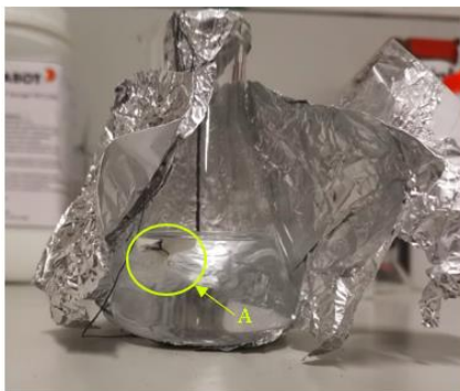
Figure 4. In vitro drug release studies (A: xerogel loaded with hydrocortisone inside the dialysis tubing).
