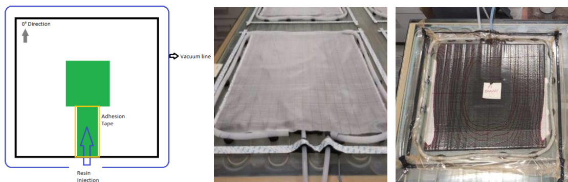
Figure 4. Representation of permeability test system set-up.
